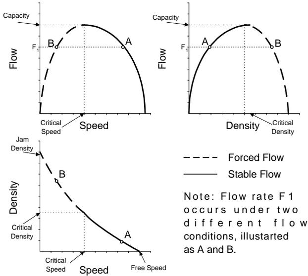
Fig. 1. The relations between flow, speed and density.
