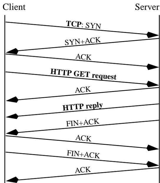
Figure 1: HTTP GET request and reply over TCP.
