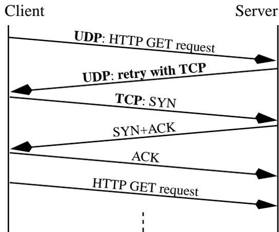
Figure 4: Explicit fall back from UDP to TCP. Server is UDP capable, but the requested resource warrants use of TCP.
