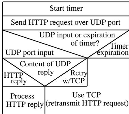
Figure 2: Algorithm executed at HTTP client application to receive HTTP service over either TCP or UDP.
