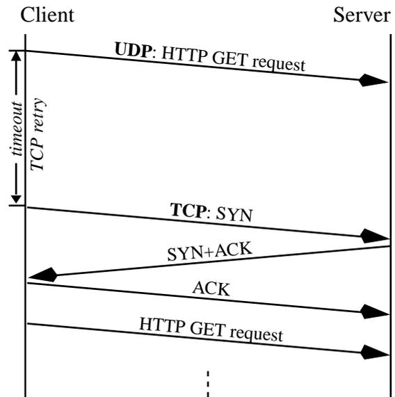
Figure 3: Implicit fall back from UDP to TCP. One of the UDP request/response packets got lost or the server is not UDP capable.
