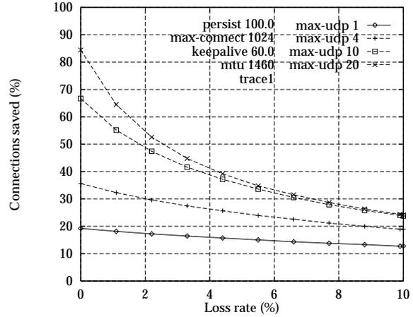
Figure 8: Effect of loss rate and max-udp parameter
